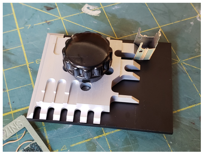
"Dry Goods Van" in progress with a photo etch metal bending tool
